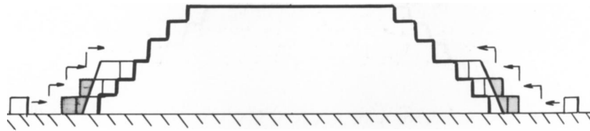
Fig. 12. Method of raising blocks to convert the stepped structure of figure 7 to one with inclined faces by the use of external steps.
